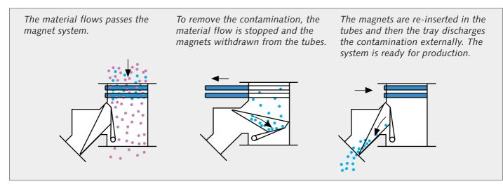
Operating principles of the Bakker Magnetics self-cleaning magnet grid.
