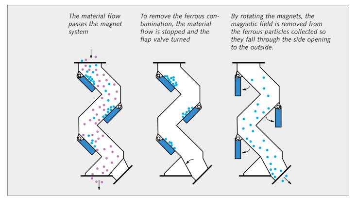
Operating principle of the Bakker Magnetics cascade magnet system.
