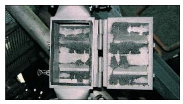
Open chute magnet in the plastics industry. The collected iron contamination is clearly visible
