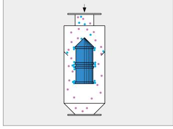
The ferrous particles extracted from the flow are collected behind the pole plates.
