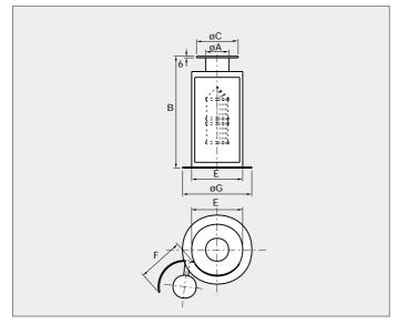
Tube magnets without outlet cone
