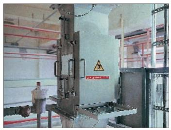
Bakker Magnetics external chute magnet in the transport system for bulk goods
