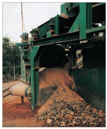
Drum magnet in use for mineral extraction
