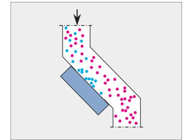
In this application, the material flow comes directly in contact with the plate magnet.
