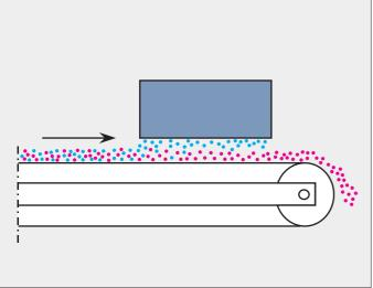
FDA plate magnets above material on a conveyor belt
