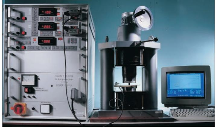
Permagraph for the analysis of the magnetic properties of material
