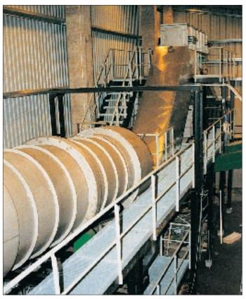
Overband magnet system in a cryogenic installation
