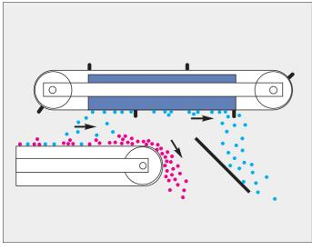
Overbelt magnet system mounted longitudinally over the end roller of the conveyor belt.
