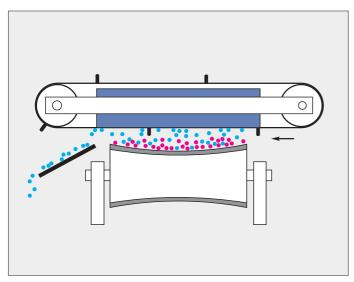
Overbelt magnet system mounted transversely over the conveyor belt.
